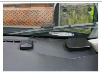
CP4 GPS and LTE antenna properly installed on the Vehicle Dash
