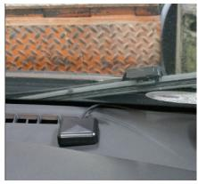
**CP4S GPS antenna properly installed on the Vehicle Dash**
