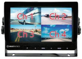
LCD Camera Channel Display order (Quad View)
