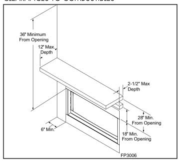
**Floor Clearance** — The fireplace may be installed directly on a combustible floor or a raised platform of an appropriate height. Do not place fireplace on carpeting, vinyl, tile or other soft floor coverings. It may, however, be placed on flat wood, plywood, particle board or other hard surfaces. Be sure fireplace rests on a solid continuous floor or platform with appropriate framing for support and so that no cold air can enter from under the firebox.
