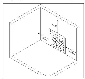
Figure 6.1 Clearance and Height Requirements
