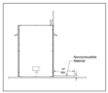
Figure 6.6 Floor Clearance Above Noncombustible Flooring Material
