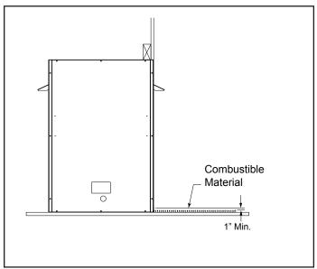
Figure 6.5 Floor Clearance Above Combustible Flooring Material
