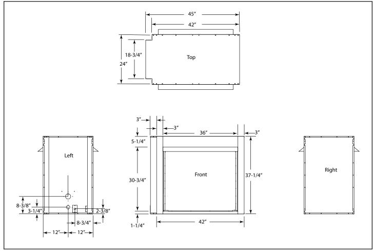
Figure 4.1 Framing Dimensions
