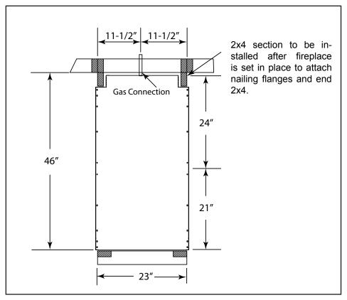
Figure 4.2 Top View of Framing Specifications
