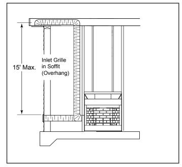
Figure 8.2 Concrete Slab Installation (Optional Outside Air Runs)
