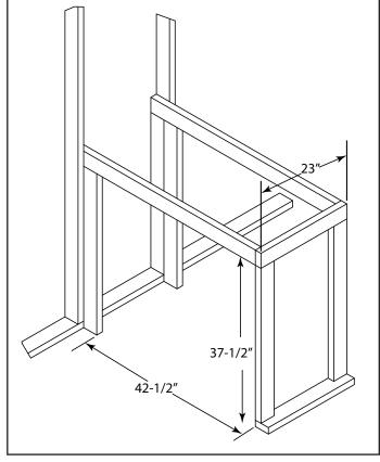
Figure 4.3 Framing Specifications
