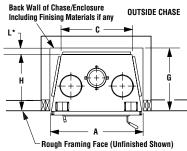
\* Zero Clearance From Back Spacer to Wall
