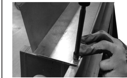
Step 2. Affix shield with 5/16" hex screws into front standoff.
