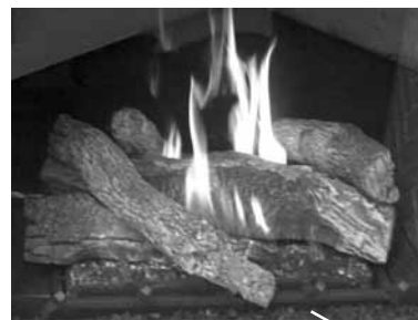
Figure 49: Burner Flame Appearance — Control Side
