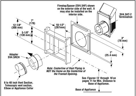
Figure 41 Installing the Square Horizontal Termination (SV4.5HT-2)
