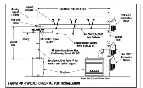
The unitized design of the **Secure Vent** components will engage and seal both the inner and outer pipe elements with the same procedure. Sealant and securing screws are not required.
