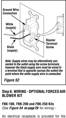
An electrical receptacie is provided for the installation of the **FBK-100**, **FBK-200** and **FBK-250** forced air blower kits. Electrical power must be connected to this receptacle in order to operate these blowers. Install the blower kits according to the installation instructions provided with the kits.
