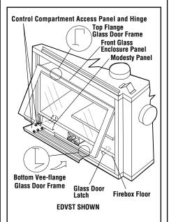
Note: When installing the glass door, ensure the spacing on both sides is even and equal.
