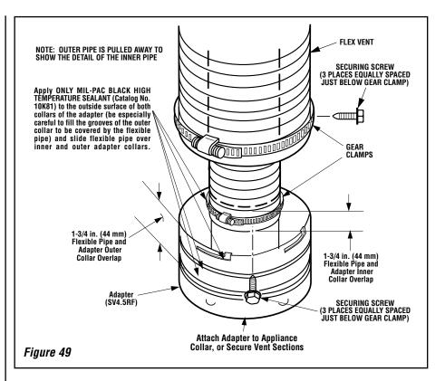
2. Apply a bead of Mill-Pac Black (700°F) high temperature sealant - Catalog No. 10K81) to the outer adapter collar; to the grooves of the collar which extend approximately 1 inch from the end and to the flat surface, approximately 1-3/8 inches from the end.
