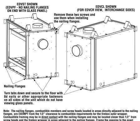
screw heads and the firebox wrapper in areas adjacent to the nailing flanges. Frame the opening to the exact dimensions specified in the framing details of this manual.
