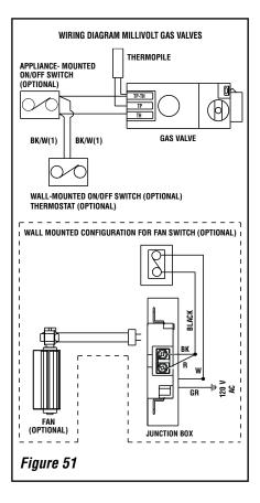
Refer to Section A for millivolt appliances and Section B for electronic appliances. The gas valve is set in place and pre-wired at the factory on both models.
