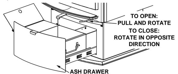
This creates a fire hazard that may result in a house/chimney fire, internal damage to the stove or discoloration to the gold plated door (plated finishes are not covered by the warranty). To ensure that the ash well is fully closed, allow the door to snap shut, dislodging anything that may be stuck at the opening.
