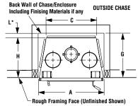
\* Zero Clearance From Back Spacer to Wall
