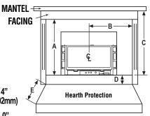
NOTE: Hearth protection to be min. 3/8" (10mm) thick non-combustible or equivalent, with a k factor of .84.
