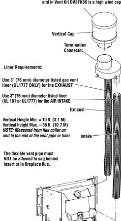
The existing fireplace chimneys may take various contours which the flexible liners will accommodate. However, keep the flexible liner as STRAIGHT as possible, avoid unnecessary bending.
