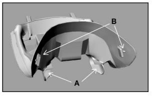
Installation Rear Install the rear seat by guiding the rear square bumper support into its receiver, then push down on the front of the seat to engage and lock the seat.
