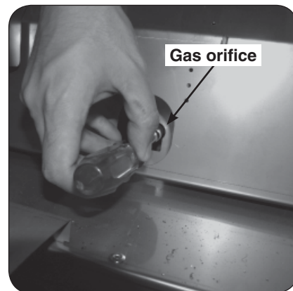
Fig. 3-2 Replace the gas orifice
