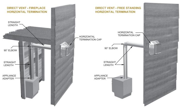
Note: Twist-Lock Pipe overlaps  $1\frac{1}{2}$ " when joined together. Therefore, assembled length on all sizes is  $1\frac{1}{2}$ " less than listed length.
