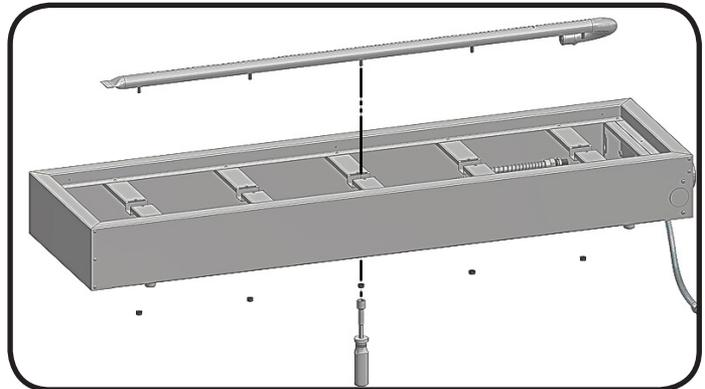
**Reinstallation:** Reverse the procedure to reinstall the burner. Check that the valve enters the burner when installing. Replace the glass embers. When the appliance is put back in service, check the burner flame pattern with the image below.
