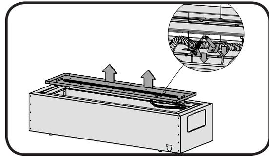
4. Disconnect the stainless steel flex connector from the orifice using (2) wrenches.
