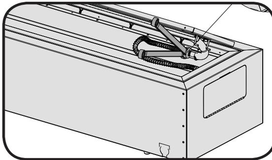
5. Unscrew the propane orifice from the inside of the burner as illustrated.
