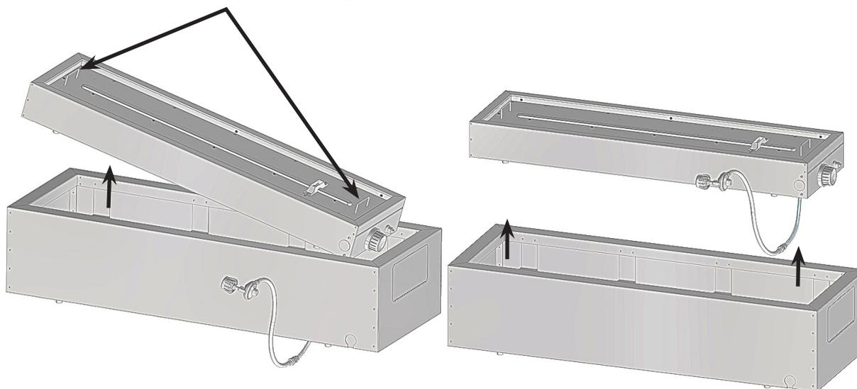
3. The supply can feed either into the side of the burner base, or is fed from below the base. The gas line needs to be disconnected from the gas valve and reconnected in order to do this. This must be done by a licensed gas fitter and the connections need to be leak tested according to the leak testing instructions before using the unit.
