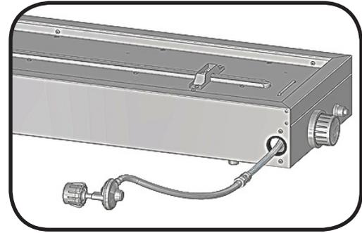
4. The burner unit can be built into a non-combustible enclosure. The control module can be removed from the burner unit and located up to 12" away from the burner unit. A cap is provided to close the opening in the side of the burner module. The gas line needs to be disconnected and reconnected in order to do this. This must be done by a licensed gas fitter and the connections need to be leak tested according to the leak testing instructions before using the unit.
