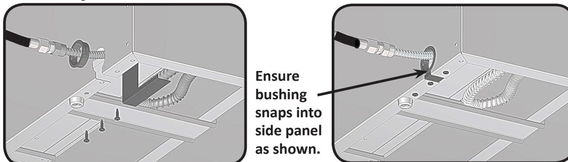
If the gas supply is to be routed through the side of the enclosure remove the (3) screws from the cover plate so the hole is exposed. Snap the bushing into the side panel to secure the hose in place. Slide the cover plate over, and reinstall.
