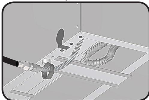
2. The burner unit can be used either with or without the enclosure. Simply lift the unit out of the enclosure to separate. A second person is required to guide out the gas hose /regulator when removing the burner unit from the enclosure. The burner unit can be placed directly on combustible surfaces, but the required clearances to the sides and top must still be maintained.
