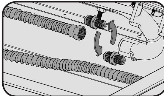
6. Replace the propane orifice with the natural gas orifice supplied.
