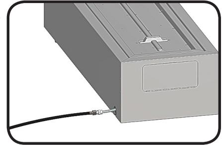
**Purge the gas supply line of any trapped air prior to the first firing of the unit.**
