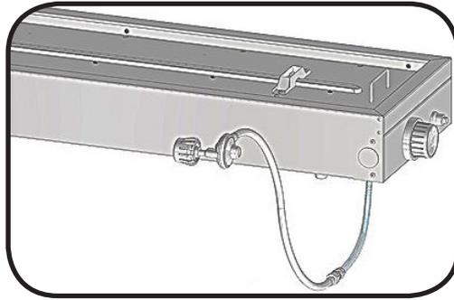
***The gas supply is shown entering the side of the burner.***
