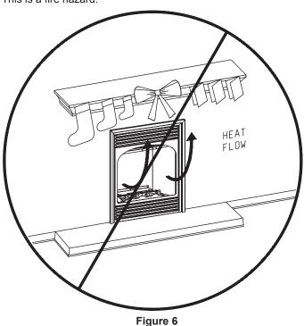
No greeting cards, stockings or ornamentation of any type should be placed on or attached to the fireplace. This is a heating appliance. The flow of heat can ignite combustibles.
