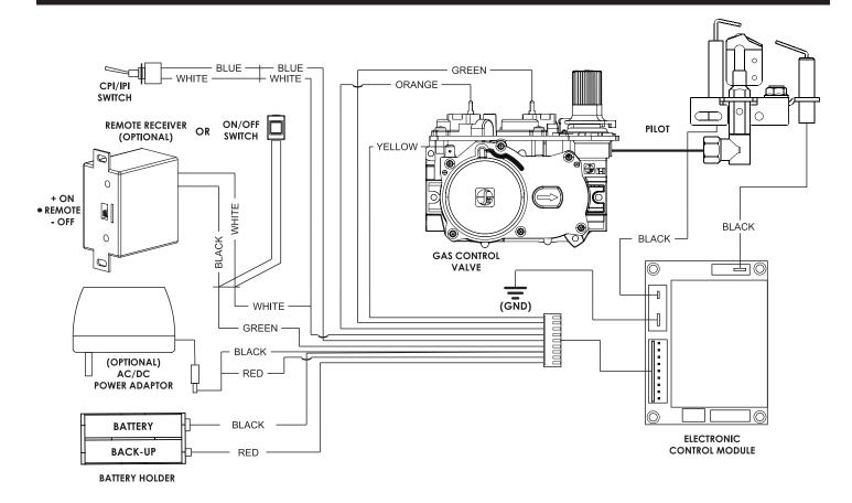
If any of the original wire as supplied with this unit must be replaced, it must be replaced with equivalent gauge and temperature rated wire.
