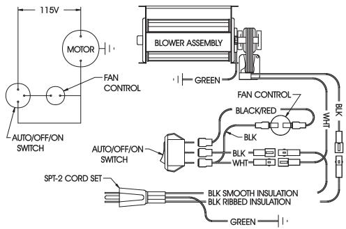
IF ANY OF THE ORIGINAL WIRE AS SUPPLIED WITH THIS UNIT MUST BE REPLACED, IT MUST BE REPLACED WITH NO. 18 GAGE  $150^{\circ}$ C 2/64 INSULATION WIRE OR ITS EQUIVALENT.
