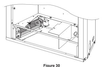
Attach black wire from wire harness to OFF terminal on AUTO/ OFF/ON switch.
