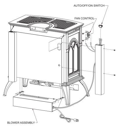
Figure 26 -VFD20CC shown
