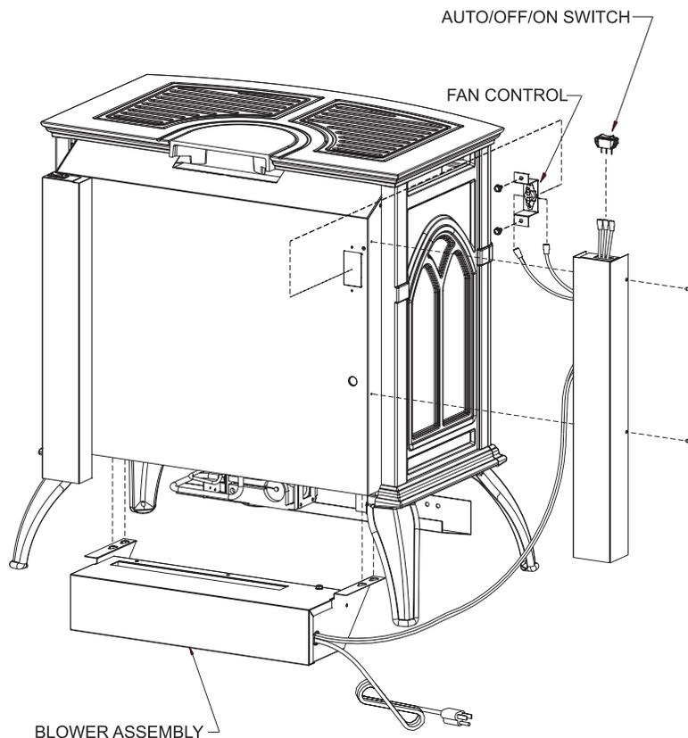
Figure 26 -VFD20CC shown
