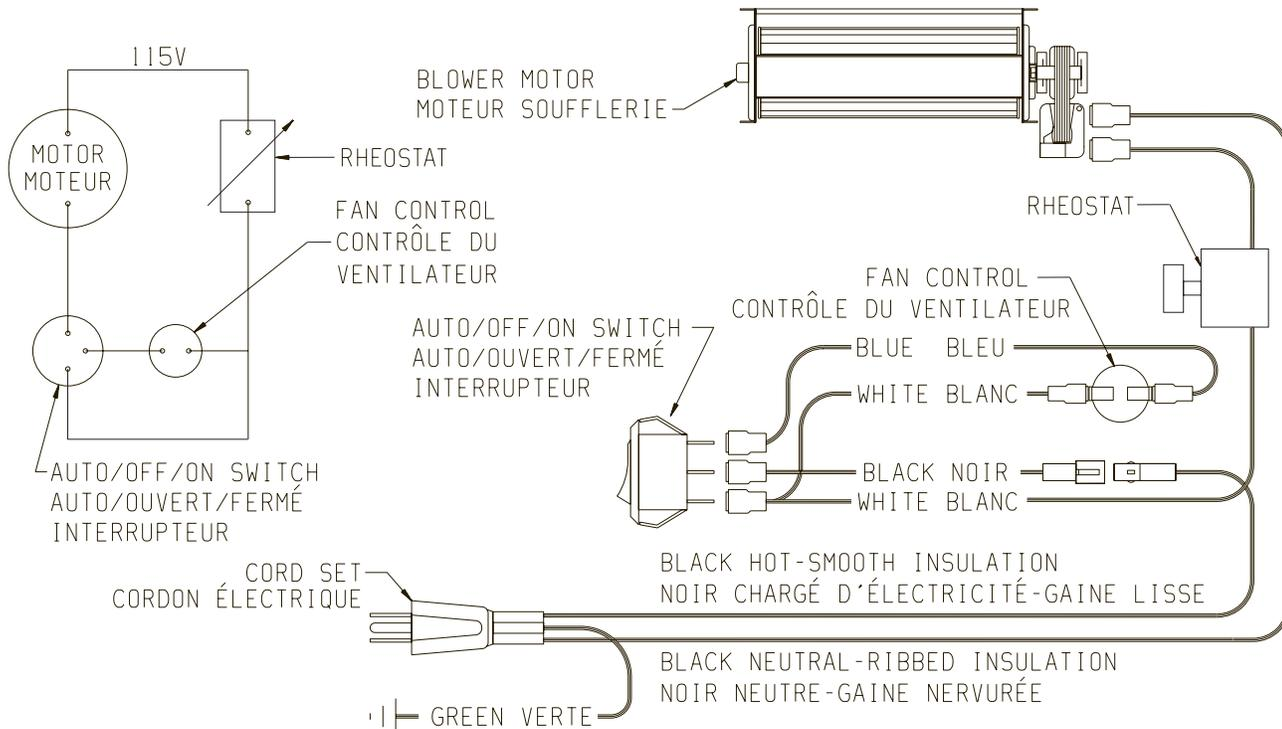
IF ANY OF THE ORIGINAL WIRE AS SUPPLIED WITH THIS UNIT MUST BE REPLACED, IT MUST BE REPLACED WITH NO. 18, 150°C WIRE OR ITS EQUIVALENT. SI UN DES FILS ÉLECTRIQUES ORIGINAUX, VENANT DU FABRICANT AVEC CETTE UNITÉ, DOIT ÊTRE REMPLACÉ, VOUS DEVEZ LE REMPLACER AVEC UN FIL ÉLECTRIQUE DE NUMÉRO 18, 150°C OU L'ÉQUIVALENT.
