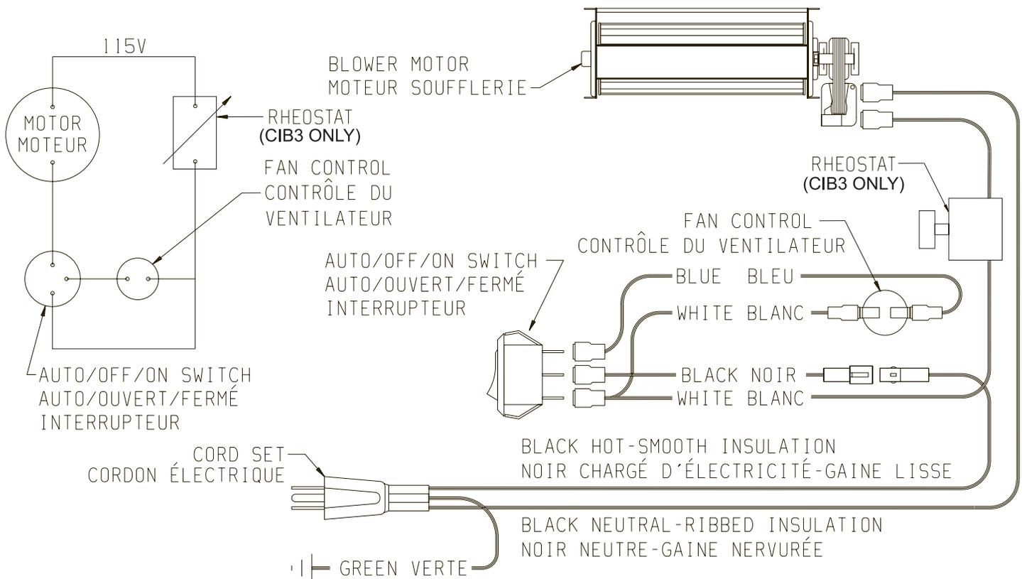
IF ANY OF THE ORIGINAL WIRE AS SUPPLIED WITH THIS UNIT MUST BE REPLACED, IT MUST BE REPLACED WITH NO. 18, 150°C WIRE OR ITS EQUIVALENT.
