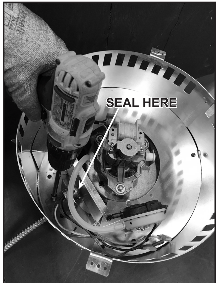
Figure 3.13 Attach Wire Harness Bracket to Bottom Dish
