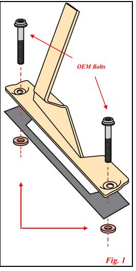
To remove the rear seat when the backrest support bracket is installed, you will need to push (or flex) the support bar forward while lifting the rear seat off the bike.
