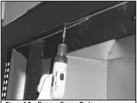
Figure 3.7 Remove Screen Rods
