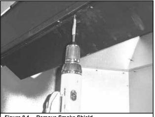
Figure 8.1 **Remove Smoke Shield**
