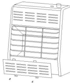
Figure 6 - Removing Lower Front Panel Of Heater
