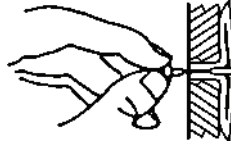
Figure 9 - Popping Open Anchor Wing For Thin Walls
