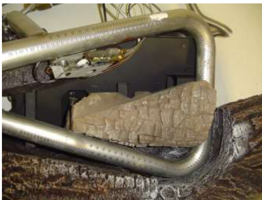
Figure 27A - Installing Charred Log Top View
