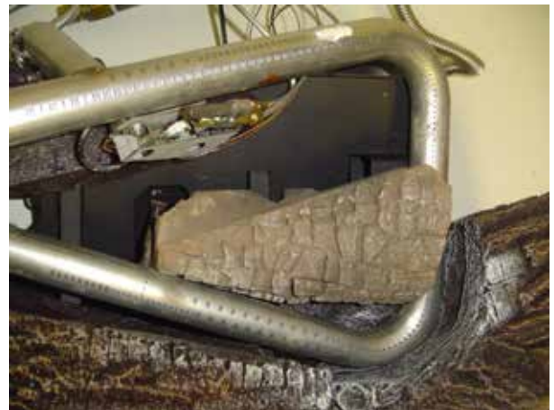
Figure 19A - Installing Charred Log Top View
