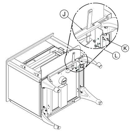
6. Put the stove on its legs, install the ash drawer included with the kit. Put back the firebricks, the ash plug and the door on the stove. See step 1.
