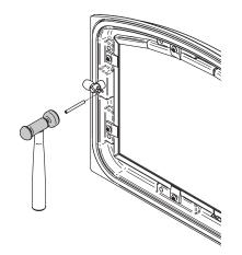
Figure 14: Installing the split pin
