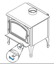
As the air intake is reduced, the flame slows down. If the flames diminish to the point of disappearing, the air intake has been reduced too early in the combustion cycle or the wood used is too wet. If the wood is dry and the air control is used properly, the flames should decrease, but remain bright and stable.
