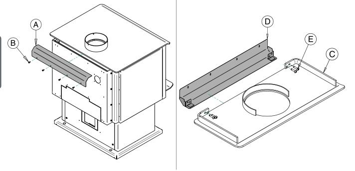
Install the step top and fix it in place using the screws (B) removed previously. 6.
