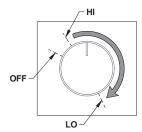
The blower has a variable speed control that can be adjusted in three different positions; either from high (HI) to low (LO) or closed (OFF).
