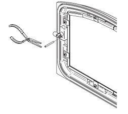
Figure 13: Removing the split pin
