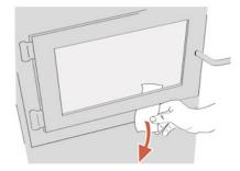
In order for the stove to burn at its best efficiency, the door must provide a perfect seal with the firebox. The tightness of the door seal can be verified by closing and latching the door on a strip of paper. The test must be performed all around the door. If the paper slips out easily anywhere, either adjust the door or replace the gasket.
