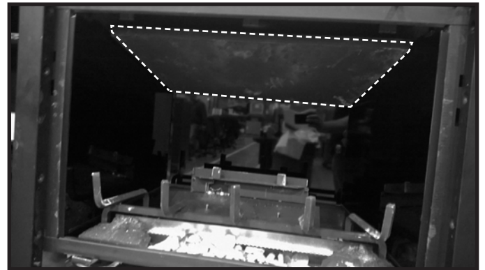
Figure 4. Install Top Refractory Panel
