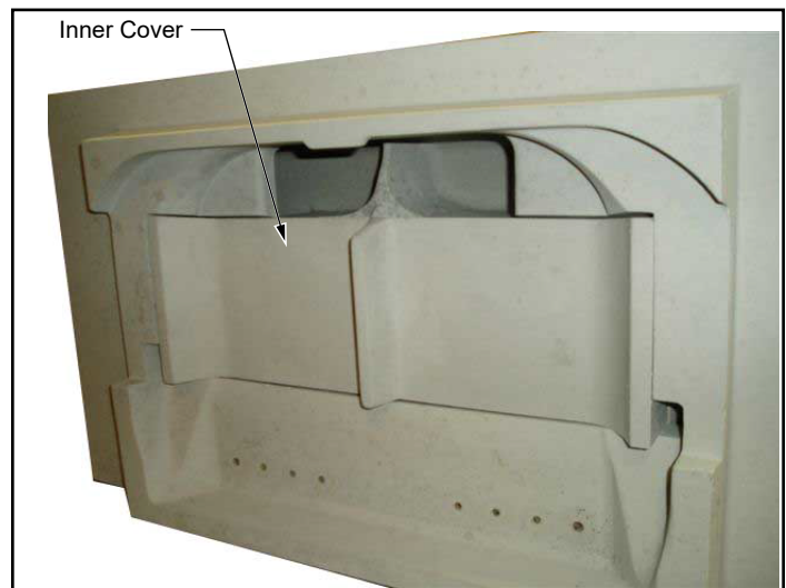
Figure 3.11 - Remove inner cover.
