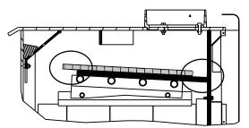
Ceramic Blanket is NOT in contact with the back of the firebox and NOT even with the Baffle Board in the front.
