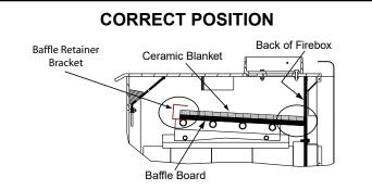
Ceramic Blanket and Baffle Board MUST be in contact with the back of the firebox and even with each other in the front.
