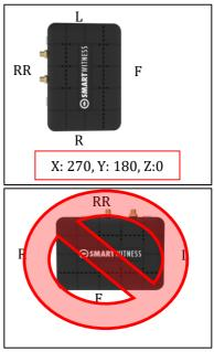
4) When device is in a sideway position with the TOP to the right
