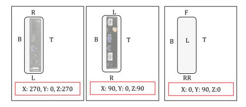
REMARK: Do no install the device with the Front facing down position.
