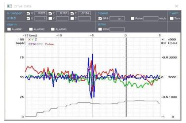
**G-Sensor:** (X axis: red, Y axis: green, Z axis: blue, based on the positioning of the main unit) is shown with the data reference point zero-point calibrated and positive shocks as (+) and negative shocks as (-).
