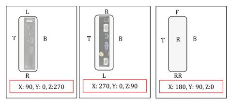
6) When device is in a sideway position with the TOP facing rear
