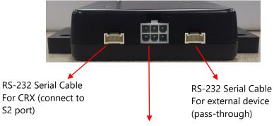
Power cable port (Power Input/Output)
