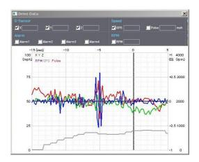
**G-Sensor:** (X axis: red, Y axis: green, Z axis: blue, based on the positioning of the main unit) is shown with the data reference point zero-point calibrated and positive shocks as (+) and negative shocks as (-).
