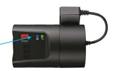
There will be a beep and LED light blink to indicate the G-Sensor calibration has registered.
