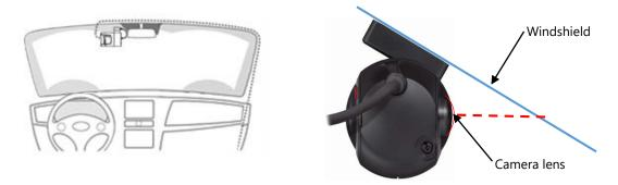
**IMPORTANT:** Make sure that the glass is clean and dry before attaching. Hold the camera in position with firm pressure for 30 seconds. The glass temperature should not be too hot or cold. Please install in moderate temperature (recommended between  $50^{\circ}F \sim 80^{\circ}F$ )
