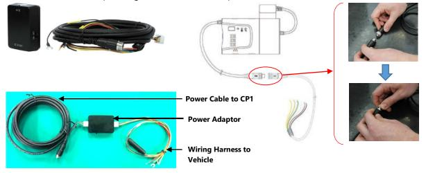
After Connecting the INT1S power cable to the CP1 power lead, lay out the power cable roughly where it will run once hidden behind the vehicle's interior panels. This gives you an idea of where to route the cable and how much slack to leave on the way down to the vehicle's power source.
