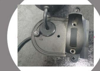
Replace the camera and screw in the screws.
