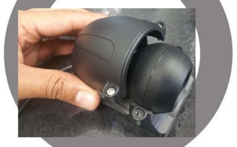
Then close the casing of the camera and screw back the screws.
