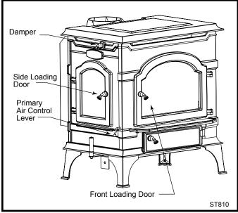
Fig. 24 The heater controls.
