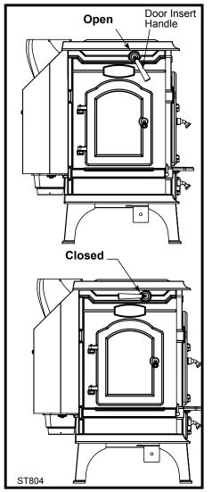
Fig. 27 Damper operating positions.
