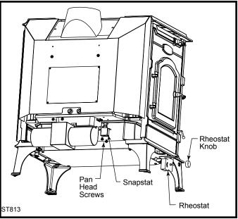
Fig. 23 Fan installation.
