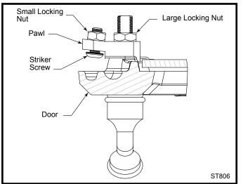
Fig. 31 Door latch adjustment.
