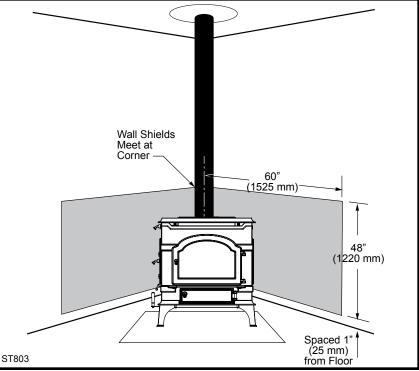
Fig. 18 Corner wall protection.
