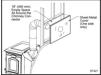
Fig. 11 Hollow wall pass-through.
