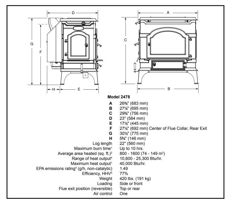
Fig. 1 Dutchwest Convection Heater specifications.
