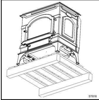
Fig. 21 Reposition stove so one rear leg can be attached.
