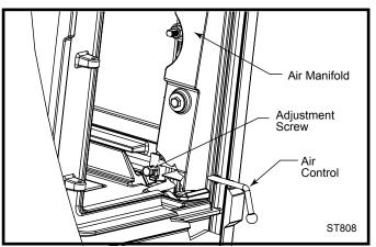
Fig. 34 Primary air control adjustment.
