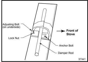
Fig. 33 Damper adjustment.
