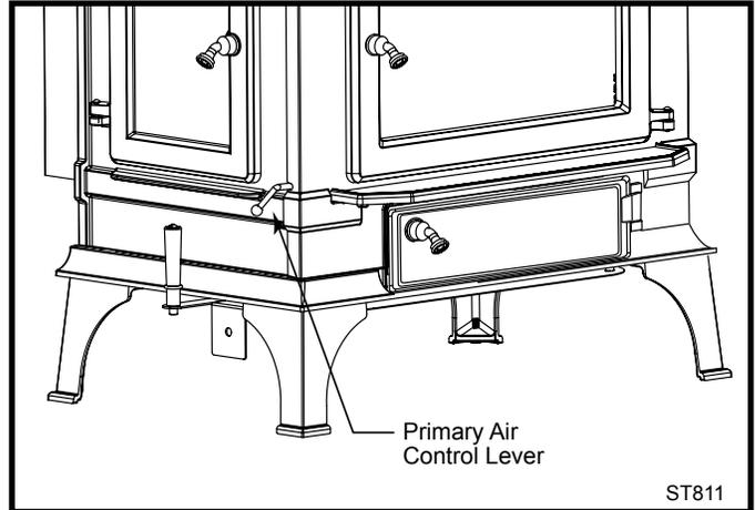
Fig. 25 Turn primary air control lever clockwise to open.
