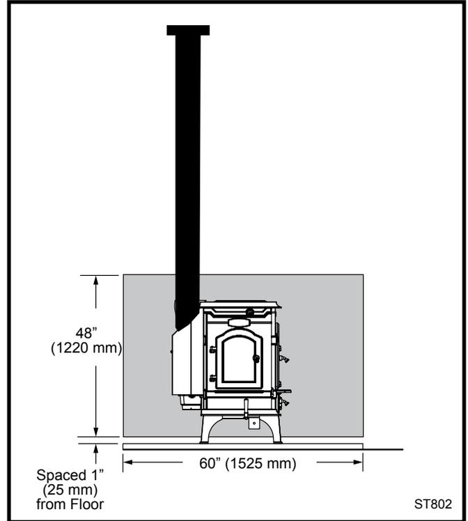
Fig. 17 Sidewall protection.
