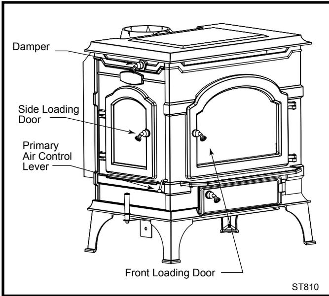
Fig. 24 The heater controls.
