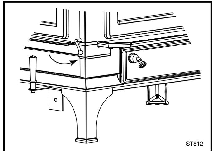
Fig. 26 Turn primary air control lever counterclockwise to close.
