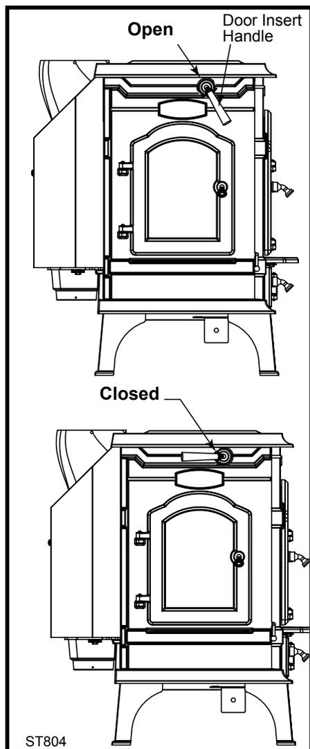
Fig. 27 Damper operating positions.
