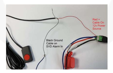
3. Once all cables have all been connected, you can now power on the SVD unit. Once powered on, press the "Menu" button on the remote and input your admin password. By default this password is "6666". Once in the main menu, head to the Alarm option and click "Sensor". You can now activate the Alarm you connected the button to. You can also rename and assign a camera to show full screen once the button is pressed.
