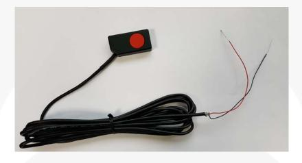
Once the Panic Button is ready, you can now connect the button to the SVD unit. On the panic button, you will have to connect the Ground (Black Cable) to an "Alarm In" on the SVD and then put the Positive (Red cable) on the Panic Button to a power source (12V). Please see the image below.
