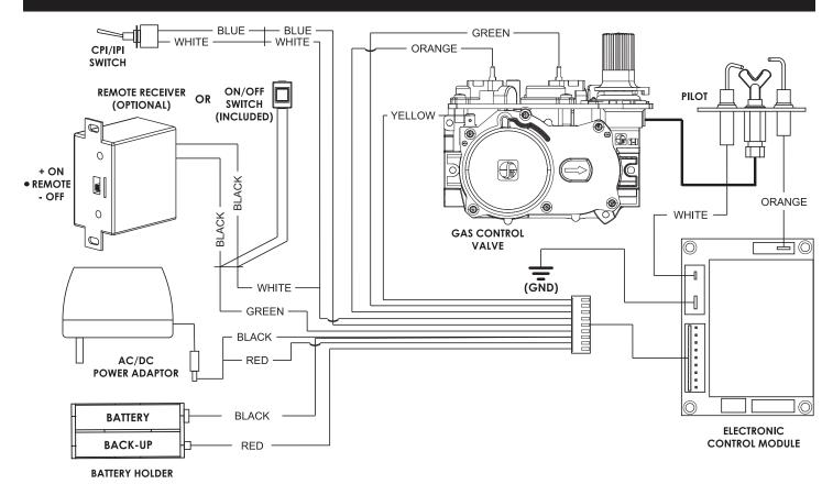
If any of the original wire as supplied with this fireplace must be replaced, it must be replaced with equivalent gauge and temperature rated wire.
