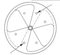
2/3 OPEN AND TWO INDICATED HOLES ALIGNED
