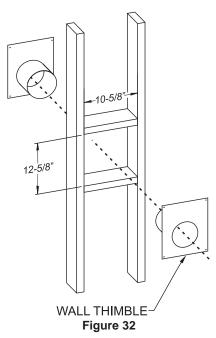
**NOTICE:** SD58DVAWTEC Wall thimble is necessary to maintain the required three inches of clearance to combustibles above the vent. Framed hole dimensions shown above are for this wall thimble.
