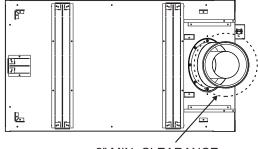
2" MIN. CLEARANCE AROUND VENT PIPE Figure 26
