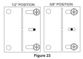
After the fireplace has been properly positioned inside the frame work, or the frame work has been built around the fireplace, the nailing flanges shall be bent 90 degrees and the fireplace should be attached to the frame work using 24 (SP) or 18 (PP) drywall screws.
