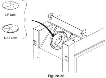
**NOTICE:** When installing NG flue restrictor, install with screws pointing in downward position.
