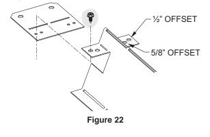
3. If necessary, the positions of the side nailing flanges can adjusted by loosening (but do not remove) the top and bottom screws, anchoring the bracket in place using a center screw from the hardware pack, and re-tightening the top and bottom screws. **See Figure 23.**
