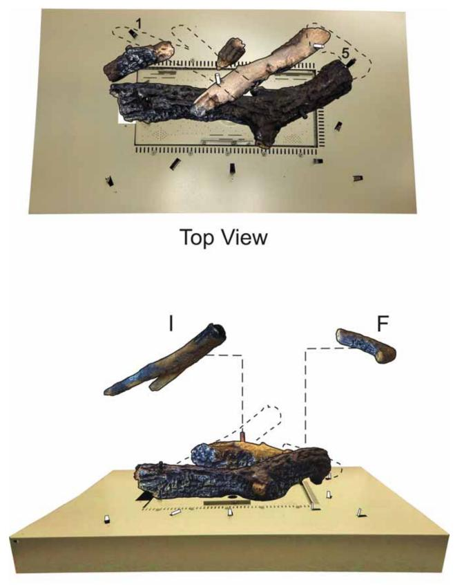
5. Place Log B onto burner tab 13 and left pin on Log A. Place Log C onto burner tab 14. Place Log K onto burner tabs 12 and 16. Refer to the images on this page.
