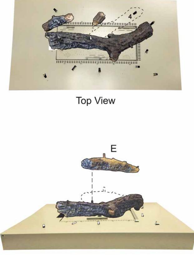
4. Place Log I onto burner tab 1 and the left pin on Log E. Place Log F onto burner tab 5 and the right pin on Log E. Refer to the images on this page.
