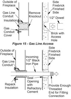
Figure 16 - Gas Line Installation
