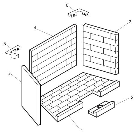
This list contains replaceable parts used in your firebox. When ordering parts, follow the instructions listed under <u>*Replacement Parts*</u> on page 23 of this manual.
