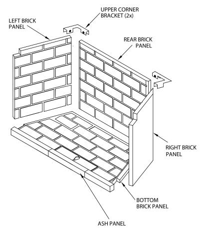
Figure 13 - Installing Refractory Panels
