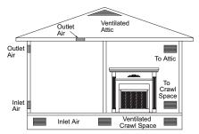
Figure 5 - Ventilation Air from Outdoors
