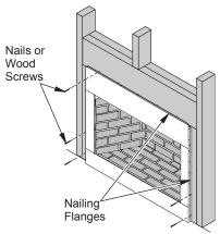
Figure 10 - Attaching Firebox to Wall Studs
