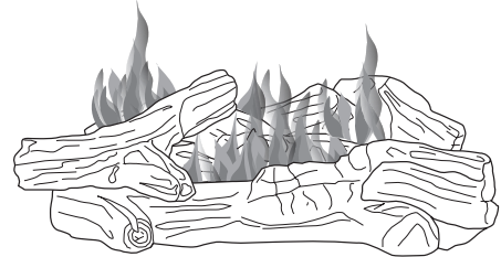
Figure 34 - Incorrect Flame Pattern with Control Knob Set to High Flame
