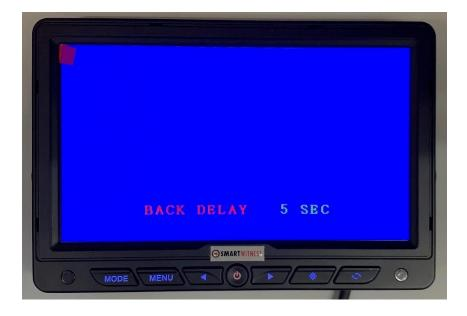
Back Delay option is only applicable with SV7QLCD-T4 model since there are total of 4 input channels. If you have cameras directly connected to the LCD-T4 monitor and are using the T4 triggers, then you may set a delay time of how long the camera channel will stay active (i.e. how long the reverse camera will stay on the monitor after the car is taken out of reverse).
