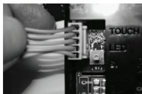
Figure 20 - Connecting end of Touch Pad Cable
