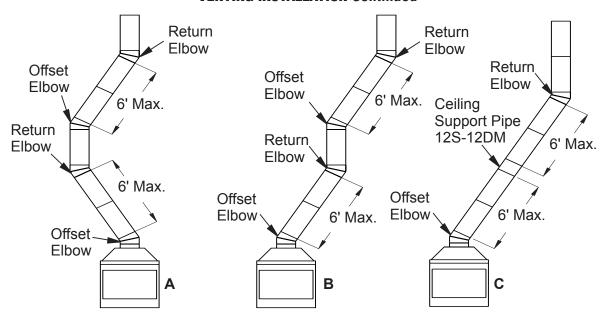
Figure 11 - Typical Offset Terminations
