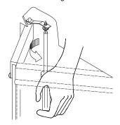
Figure 32 - Adjusting Bi-Fold Doors
