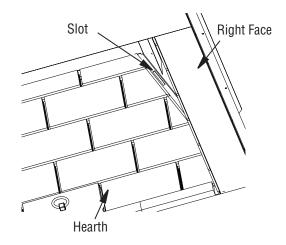
Figure 21 - Slots for Firebrick Walls
