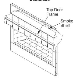
Figure 29 - Installing Top Door Frame
