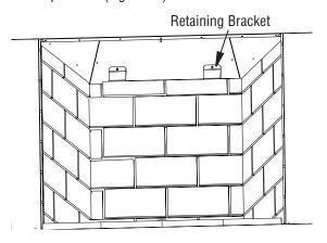
Figure 23 - Installing Rear Wall
