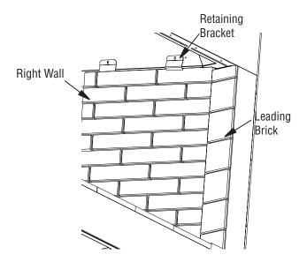
Figure 22 - Installing Side Walls
