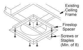
Figure 12 - Firestop Spacer with Living Space Above Ceiling
