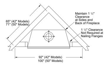
Figure 4 - Corner Installation
