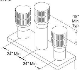
Figure 18 - Multiple Chase Installation
