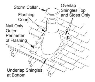
Figure 15 - Flashing Installation
