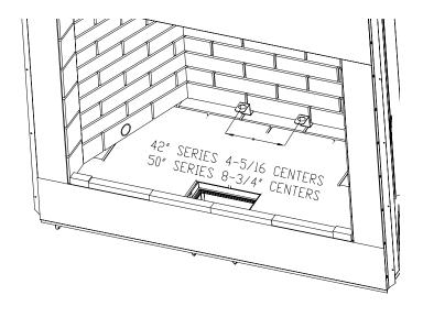
Figure 25 - Installing Grate Retainers
