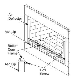
Figure 30 - Installing Bottom Door Frame and Air Deflector
