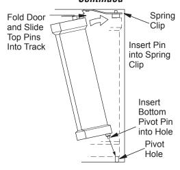
Figure 31 - Installing Bi-Fold Doors
