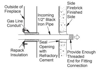
Figure 27 - Gas Line Installation
