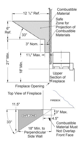
Figure 6 - Mantel Clearances to Combustible Material
