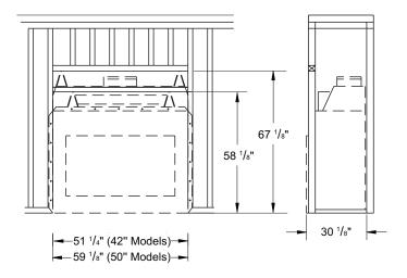
Figure 3 - Framing Dimensions
