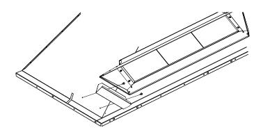
Figure 28 - Installing PureFire Hood
