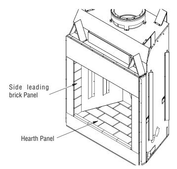
Figure 20 - Installing Hearth and Leading Brick panels
