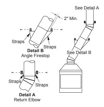
Figure 10 - Ceiling Support Pipe 12S-12DM
