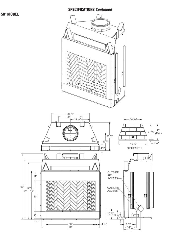
Figure 2 - 50" Models WRT6850RS, WRT6850IS, WRT6850RH and WRT6850IH
