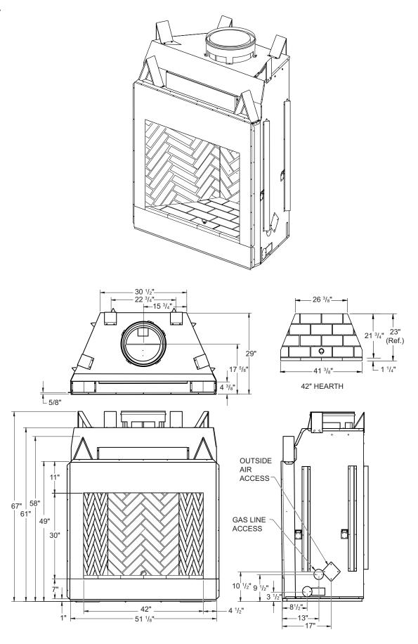
Figure 1 - 42" Models WRT6842RS, WRT6842IS, WRT6842RH and WRT6842IH
