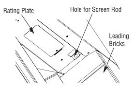
Figure 24 - Installing Fireplace Screen
