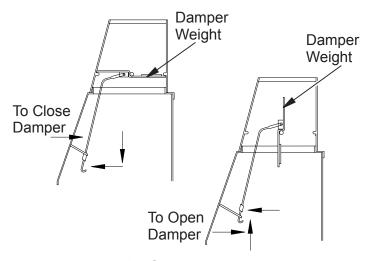
Figure 34 - Operating Damper Handle
