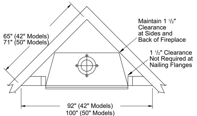
**Figure 4 - Corner Installation**
