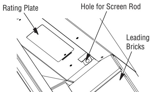
**Figure 24 - Installing Fireplace Screen**
