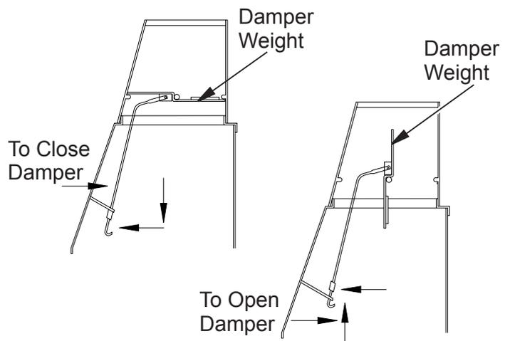
**Figure 34 - Operating Damper Handle**
