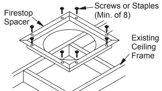
**Figure 13 - Firestop Spacer with Attic Space Above Ceiling**
