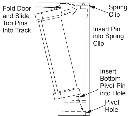
**Figure 31 - Installing Bi-Fold Doors**
