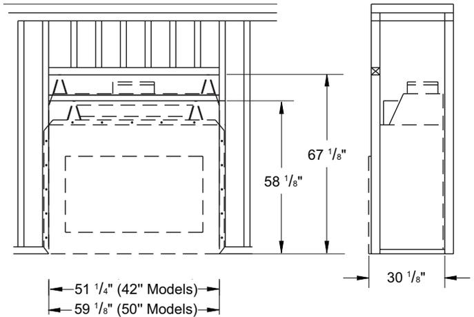
**Figure 3 - Framing Dimensions**
