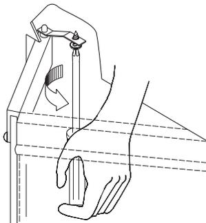
**Figure 32 - Adjusting Bi-Fold Doors**
