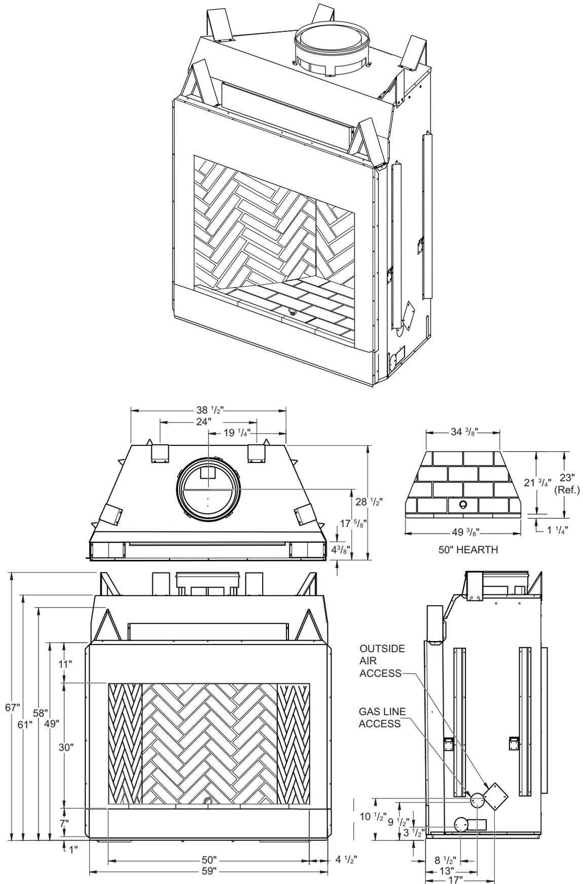
Figure 2 - 50" Models WRT6850RS, WRT6850IS, WRT6850RH and WRT6850IH
