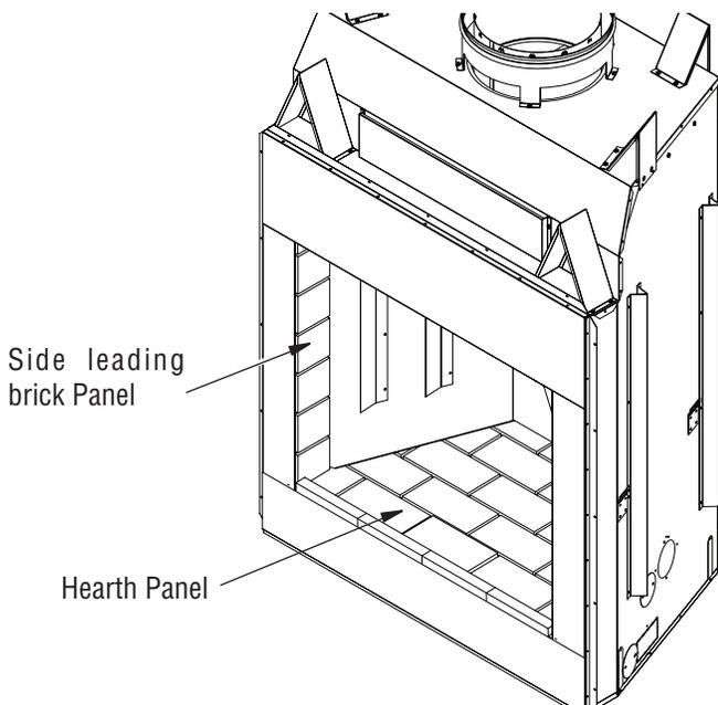
**Figure 20 - Installing Hearth and Leading Brick panels**
