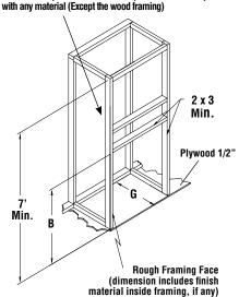
Total depth is 25 inches including the back spacer minus 1/2 inch for drywall to be flush with the facing.
