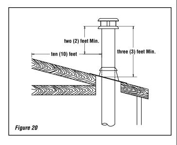
**NOTE:** 2" clearance to combustibles around chimney components required.
