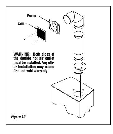
When installing the double outlet system, the hot air outlets can be installed in the same room as the fireplace, or one or both of the outlets can be installed in adjacent or upper rooms. Installing the ducts at different elevations will tend to exhaust more heat out of the higher outlet (*Figure 16*).
