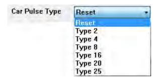
Before using "Car Pulse Type", connect the White (Speed pulse) cable to the speed pulse line on your car. Please consult your car manufacturer or a car repair shop regarding this connection.
