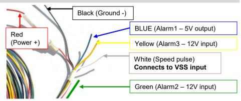
8) Make sure vehicle ignition is off and keys are out, then connect RED power (+) cable to vehicle fuse that is powered with ignition (i.e radio). Connect Black Ground (-) to car chassis.
