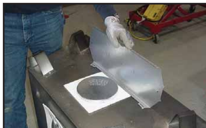
Figure 6.6 Rotate the top heat shield to the vertical position as shown above. The heat shield must remain in the vertical position.
