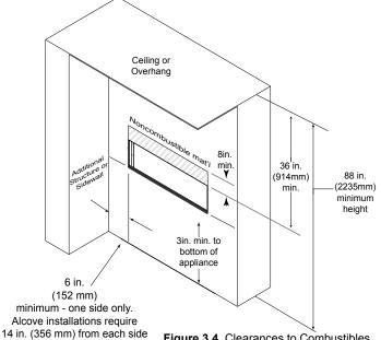
14 in. (356 mm) from each side of the firebox opening. **Figure 3.4.** Clearances to Combustibles
