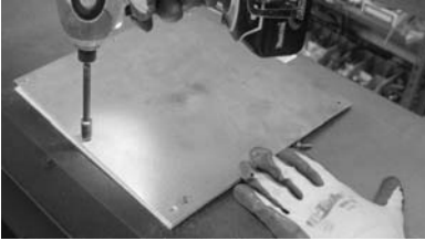
Step 1: Remove the eight (8) screws holding the top vent cover plate and gasket.
