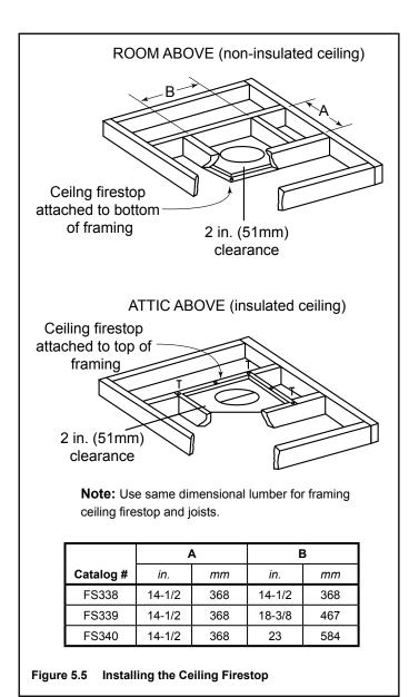
**WARNING!** Risk of Fire! DO NOT seal area between firestop opening and chimney pipe except where they enter the attic or leave the warm air envelope of the home (use 600° F sealant).
