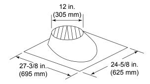
**RF370 Roof Flashing**
