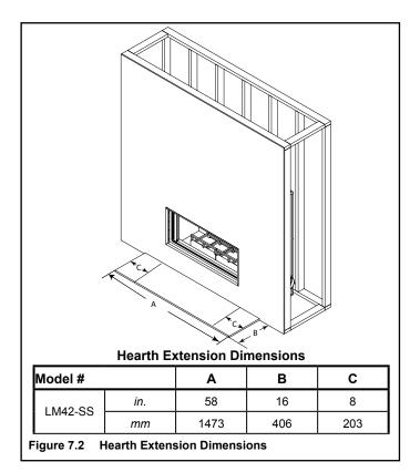
1. If the hearth extension is more than 12 inches below the fireplace opening an insulation barrier is not required but must be made of tile, stone, or other non-combustible material.
