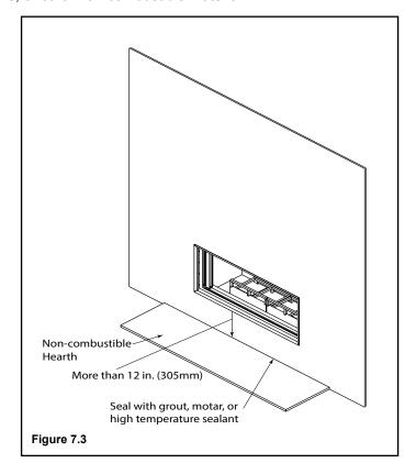
2. If the hearth extension is flush or less than 12 inches below the fireplace opening, the structure must be made of all non-combustible material (such as metal framing or equivalent material) and sitting on 1/2 in. Micore or other material with an R value of 1.03.
