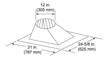
RF371 Roof Flashing
