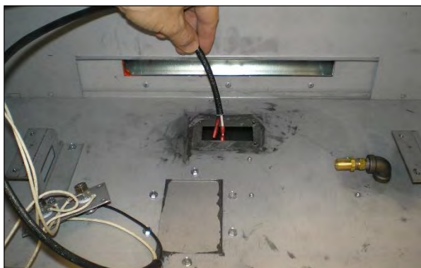
STEP 2: Insert lamp wires through access hole in firebox as above. Apply new sealant (Mill-Pac). Secure Lamp Plate with screws.
