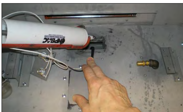
STEP 2: Insert lamp wires through access hole in firebox as above. Apply new sealant (Mill-Pac). Secure Lamp Plate with screws.
